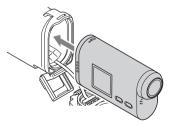
4 Insert the tab of the case cover into the slot of the case body.
