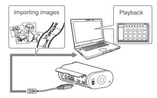
• Use the micro USB cable (supplied) when connecting the camera to your computer.
