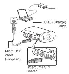
3 When charging is finished, delete the USB connection between the camera and the computer (page 44).
