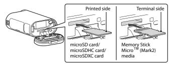
Insert the memory card properly, confirming each side is facing the correct direction.
