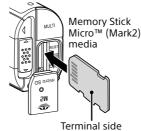
Insert the memory card properly, confirming each side is facing the correct direction.
